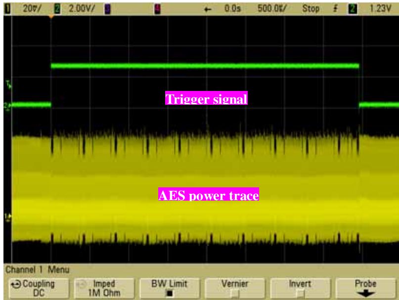
Fig 14. Sample power trace of AES operation in IC card
