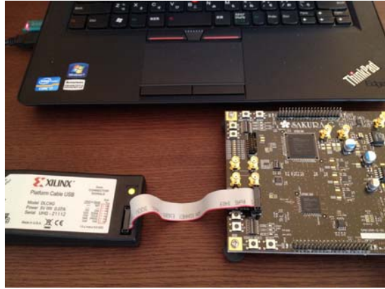
Fig. 3 Configuration cable attached to a JTAG connector of the control FPGA.
