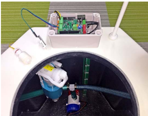
Fig. 4 A compact planter with sensor module.
