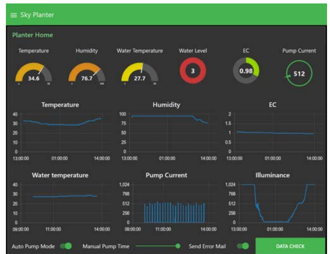
Fig. 10 Dashboard for data monitoring and pump control.
