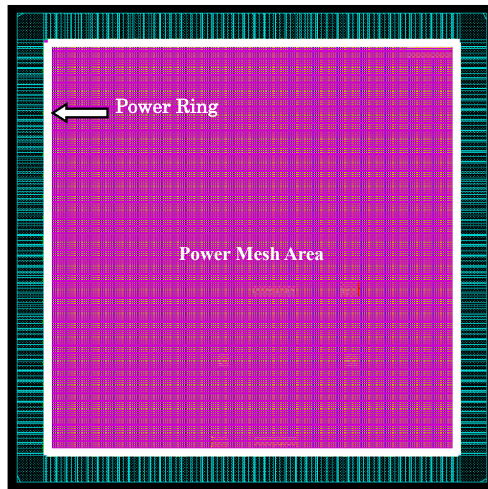
Figure 4.15 Power Wiring of the 90-nm LSI
