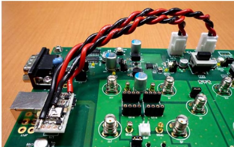
Figure 4 USB power supply circuit experimentally implemented on the SASEBO-GII
